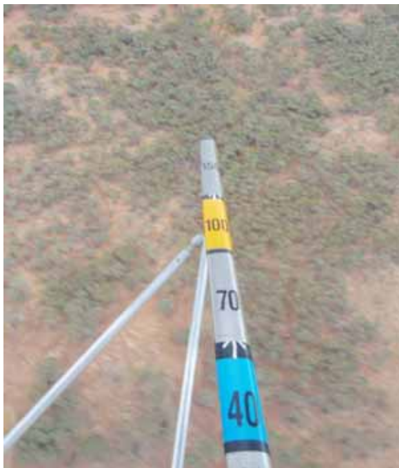
Photo 1 – Distance classes marked on aluminium boom attached to the helicopter for macropod surveys
