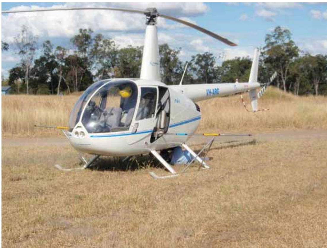
Photo 2 – Robinson 44 helicopter fitted with aluminium booms and rear doors removed
