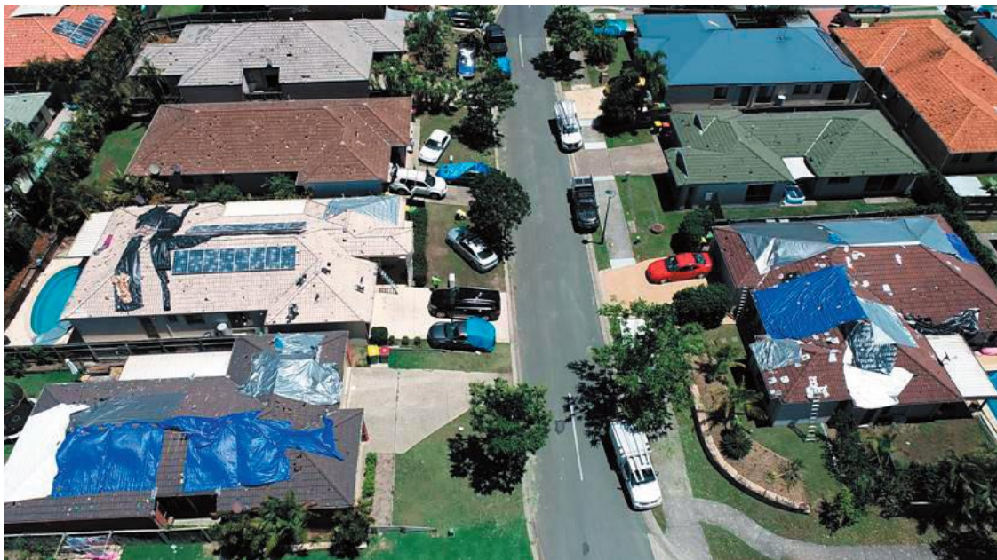
Figure 73: Damage to houses in Springfield, Queensland following a hailstorm on 31 October 2020, where hail in excess of 100mm in diameter was recorded. The damage caused to tile roofs was far greater than the damage to metal roofs, which experienced negligible damage in comparison. Source: QFES.
